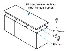
Attach the countertop at the front, center and back as shown above. When doing so, keep a longitudinal distance of 600 mm between the various fastening points. Pre-drill the holes in the top of the cabinet so that the top has room to expand and contract. If the base cabinets do not have a top, you can use the angel iron with slotted holes. If required, you can influence the direction in which the wood can work freely by giving less play to the back instead of the front.
