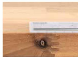
Surface disturbance: tactile knots in the wood
