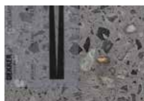
Surface disturbance: palpable pitting and surface disturbances
